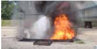
F-500 EA vs. water fire tests
